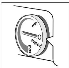
We recommend setting the thermostat on positions towards **max** only in case you want to accelerate cooling, as for example before loading smaller amounts of fresh foods or when the operation mode shall correspond to
